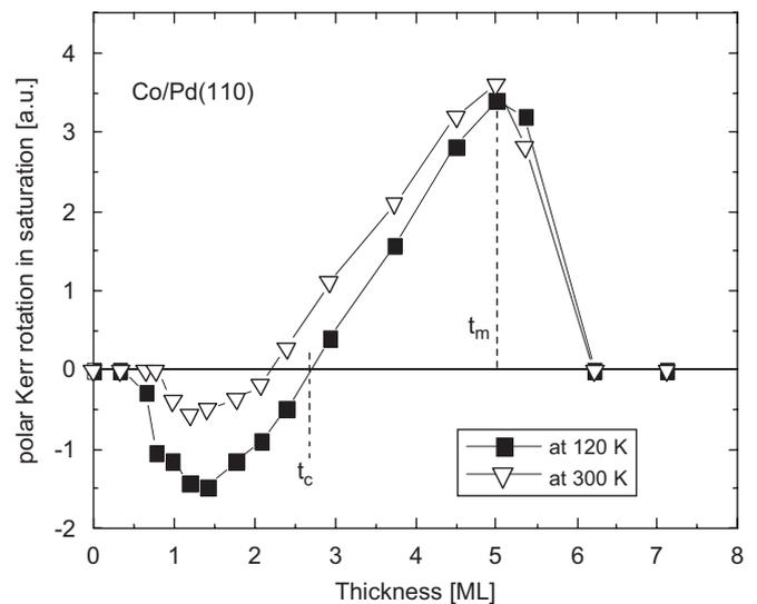
Fig. 3. Polar Kerr rotation in remanence at 120 K and at room temperature versus film thickness for Co/Pd(110) covered with Au.
