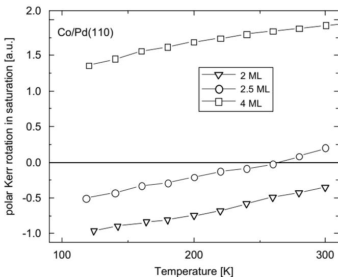
Fig. 2. Temperature dependence of polar Kerr rotation in remanence for 2, 2.5 and 4 ML thick Co films grown on Pd(110) and covered with Au.
