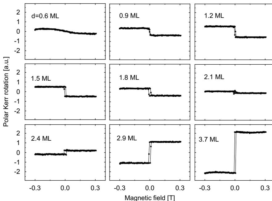
Fig. 1. Polar MOKE rotation loops measured at room temperature for Co films of different  $d$  grown on Pd(110) and covered with Au.
