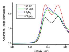
The pre-edge peak in the oxygen K edge XANES spectra of the 16h milled 1h air annealed (16h air) sample and the 16h milled 1h vacuum annealed (16h vac.) sample together with the reference spectra of magnetite and hematite.
