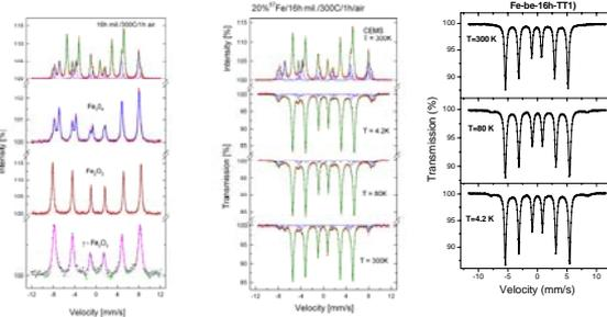
The <sup>57</sup>Fe CEMS spectra of the air annealed sample show 55% metallic iron, 34% magnetite, 8% hematite and 3% maghemite in the outer layer of 300-500nm, i.e. the CEMS probing depth.
