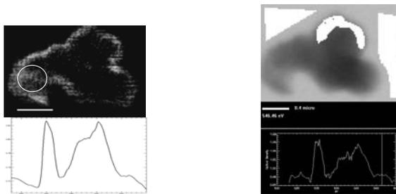
Scanning Transmission X-ray Microscopy results. Top: Oxygen map of a grain of the as cast powder. The oxygen K-edge spectrum (bottom) was integrated over the marked flat area. The pre-edge peak shape shows that the oxide is magnetite-like.
