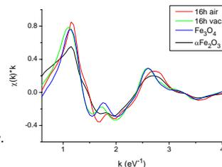
The XAFS TEY spectrum at the Fe:K edge, which corresponds to about 300 nm probing depth (similar to CEMS), shows 45% metallic Fe, 42% magnetite and 13% hematite in the layer of such a thickness.
