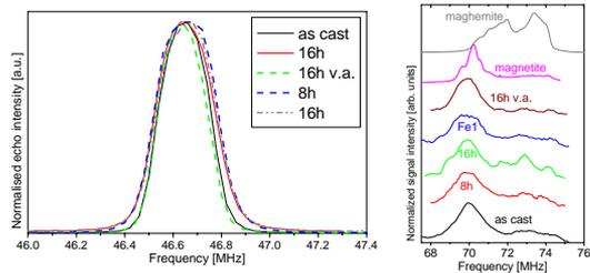
The <sup>57</sup>Fe NMR spectra at 4.2K corresponding to the iron core (left) and the oxide shell (right) for various samples.
