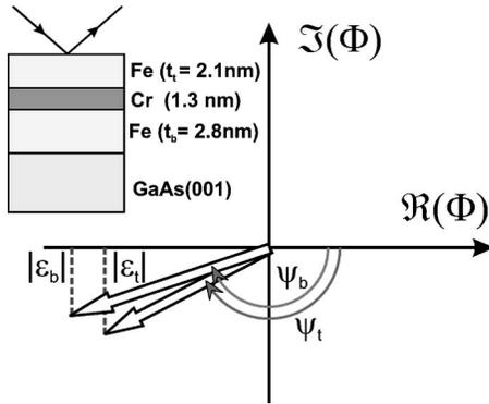
FIG. 4. Contributions of the individual top ( $t$ ) and bottom ( $b$ ) Fe layers to the complex longitudinal Kerr effect  $\Phi$  in the system Fe(2.1 nm)/Cr(1.3 nm)/Fe(2.8 nm)/GaAs(001). The vertical dashed lines marked as  $|\epsilon_t|$  and  $|\epsilon_b|$  indicate, respectively, individual contributions of the top and the bottom layers to the overall Kerr ellipticity signal calculated for the positive orientation of magnetization in both Fe layers.
