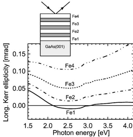
FIG. 6. Individual contributions to the longitudinal ellipticity signal in the structure Fe4/Cr/Fe3/Cr/Fe2/Cr/Fe1/GaAs(001). The thicknesses of all Fe layers are 15 ML (2.15 nm) and thicknesses of all Cr layers are equal to 9 ML (1.3 nm). The angle of incidence of the *s*-polarized photons is 49°.
