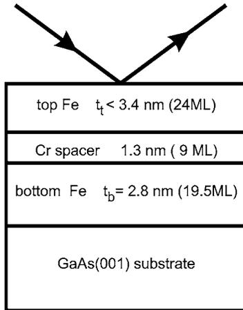
FIG. 1. A structure of the studied specimens.
